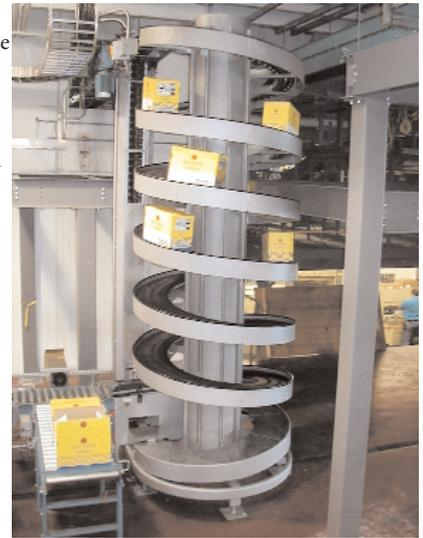
occurs when products need extra time for cooling, drying, or curing. This configuration also provides dynamic accumulation to facilitate shorter production and packaging line interruptions.
